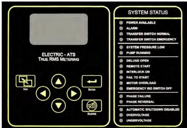
**Description** – Firetrol® FTA1000 Full Voltage Fire Pump Controllers are intended for use with electric motor driven fire pumps where the capacity of the power source permits full voltage starting. Full voltage is applied to the motor as soon as the controller is actuated. The controller monitors, displays and records fire pump system information.
